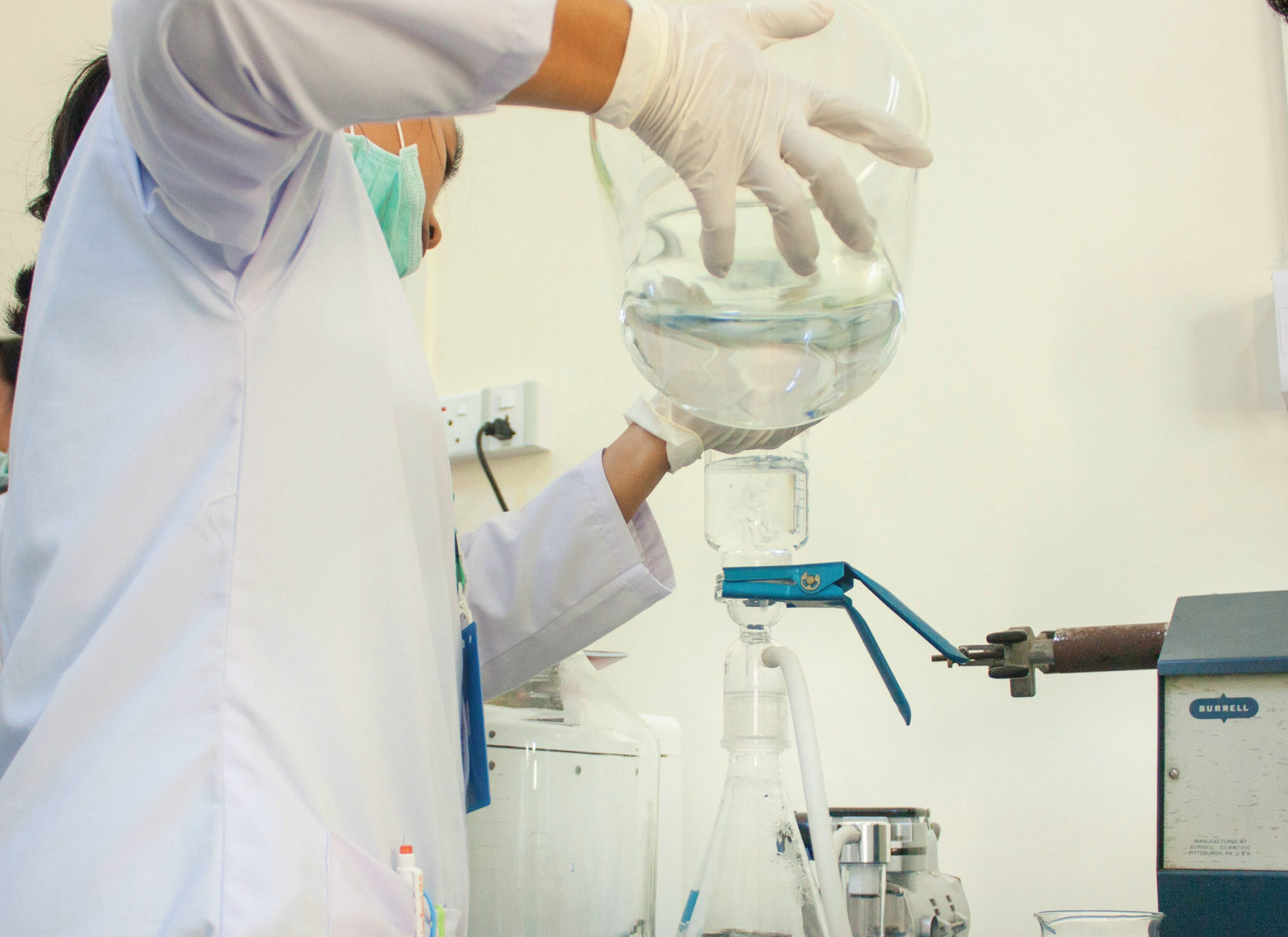
New staff at DFDA prepare reagents for dissolution testing. Photo credit: Dr. Lu Lu Kyaw/ PQM
