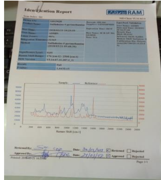
Figure 2: Falsified sulfadoxine-pyrimethamine detected by LNCQ using handheld Raman spectrometer
